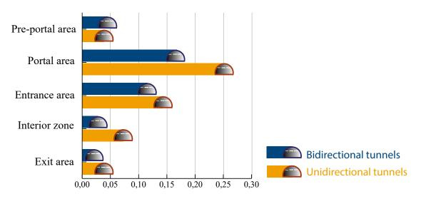
Illustration 4 : collision rates (collisions with casualties per 1 million vehicle km) in different tunnel zones in austrian motorway tunnels [34]
