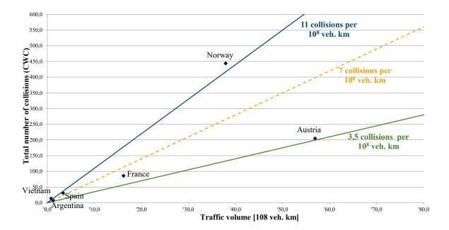
*Illustration 6: total number of collisions in the records shown in relation to the corresponding traffic for various countries – reference line for collision rates in bidirectional tunnels*
