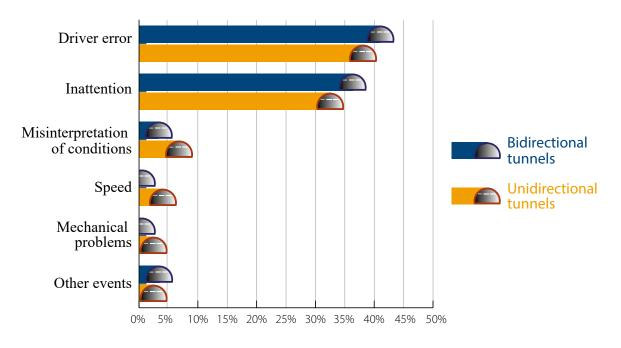
Illustration 5 : causes of collisions in austrian motorway tunnels [34]
