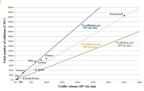
*Illustration 7: total number of collisions in the records shown in relation to the corresponding traffic for various countries – reference line for collision rates in unidirectional tunnels*
